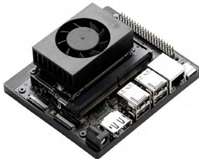
Figure 3: The Nvidia Jetson Orin Nano 8GB. This is currently the smallest embedded device that is able to run LLMs locally.
